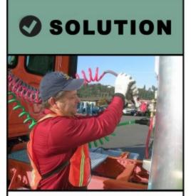
Use a full-fist power grip to make connections. Disperse force between both arms and align grip with body. Support tightening or loosening motions with your free hand.
